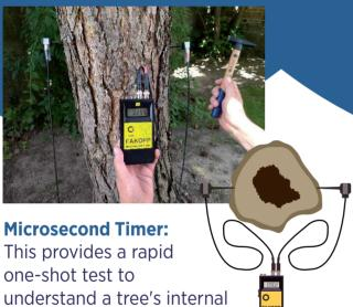
This provides a rapid one-shot test to understand a tree's internal condition. This single-shot system detects internal decay and features such as cracking, delamination or shake. The results are shown instantly or emailed to you via the App.
