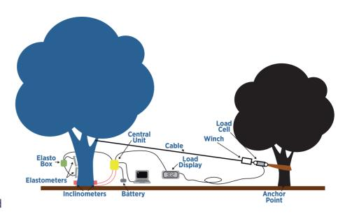
Whereas the 'Elasto Test' provides information on stem compression and tension using very accurate Elastometer's to provide information on a tree stem's resistance to fracture.
